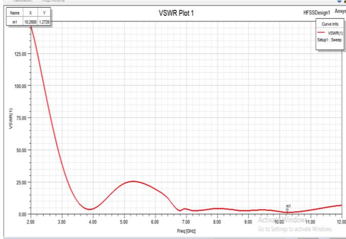
Fig 6: The standing wave ratio is obtained at 10.2GHz as 1.27726.
