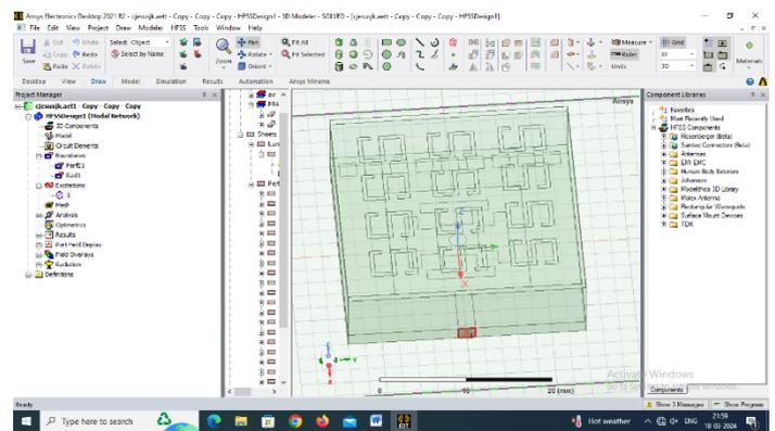
Fig 4 :Excitation assignment to the microstrip feed.
