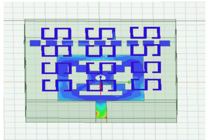
Fig 9:Field Distribution of the proposed structure
