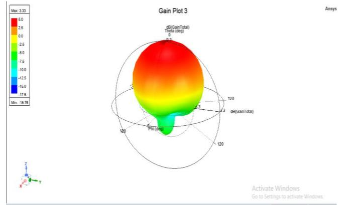
Fig 8: 3-D radiation pattern of the proposed antenna
