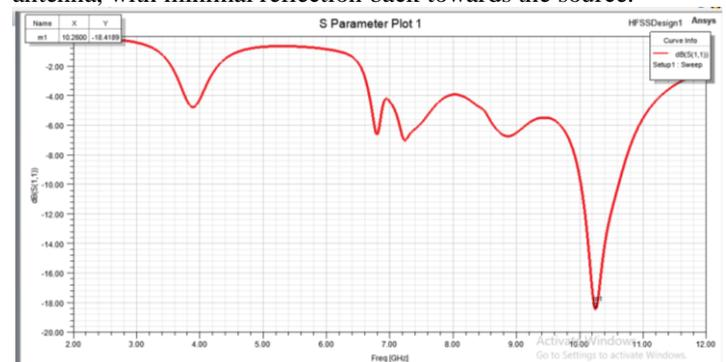
Fig 5: From this graph we have inferred that the return loss is -18.4dB which is obtained at the frequency of 10.2GHz.
