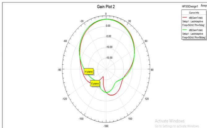
Fig7:The E plane and H plane radiation pattern meaurments of the designed antenna is given above.
