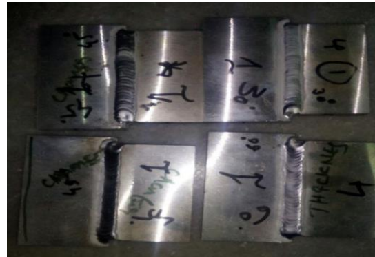
Fig 3. joining of weld plates by Tig welding
