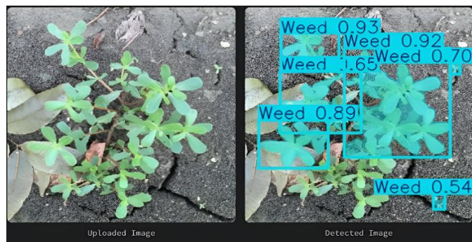
Fig. 1. Input image and YOLOv8-based weed detection output
