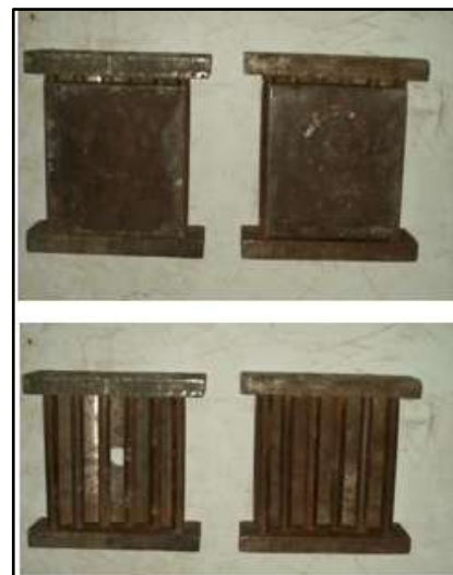
Fig. 4 Column Boundary Conditions Assembly using Teflon Sheet Plates
