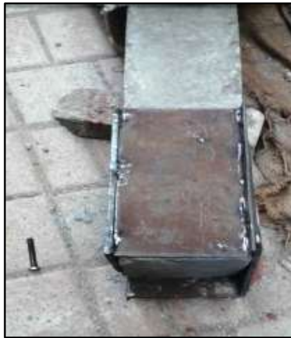
Fig. 2 Top and bottom assembly for column testing
