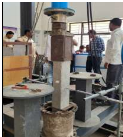
Fig. 10 Testing arrangement for the column under biaxial loading.
