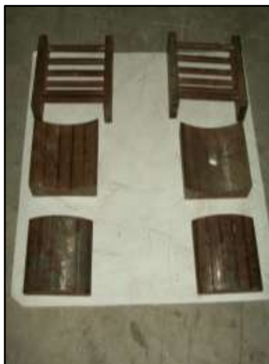
Fig. 4 Column Boundary Conditions Assembly using Teflon Sheet Plates
