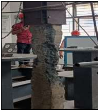
Fig. 11 Failure of the column under eccentric loading.
