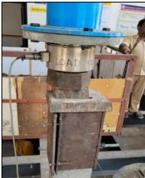
Fig. 5 Top Plate Provision for Loading
