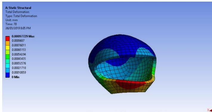
Fig. 2 Over-all Buckle of helmet due to compression
