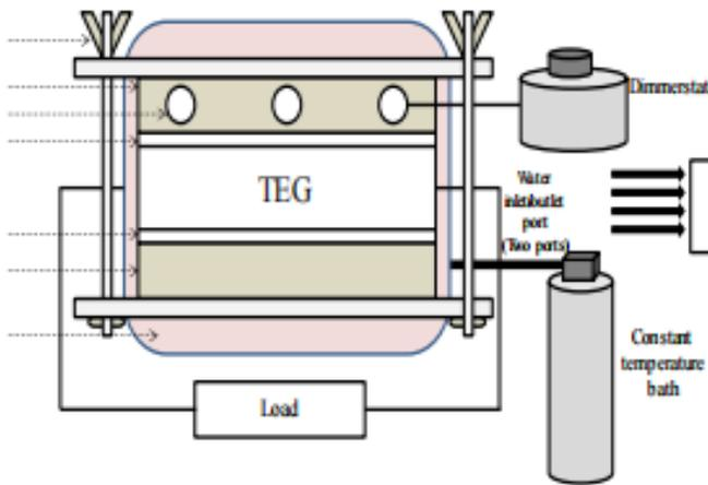
atmosphere. A constant temperature bath is used to maintain the water temperature constant at 30°C. A rheostat is connected as an external load to the hybrid TEG module to measure the output voltage and current of the module by varying the load resistance,  $RL$  between 0 to  $2\Omega$ . The required data were recorded using a data acquisition unit for further processing. The schematic diagram of the test section is given in Figure3.
