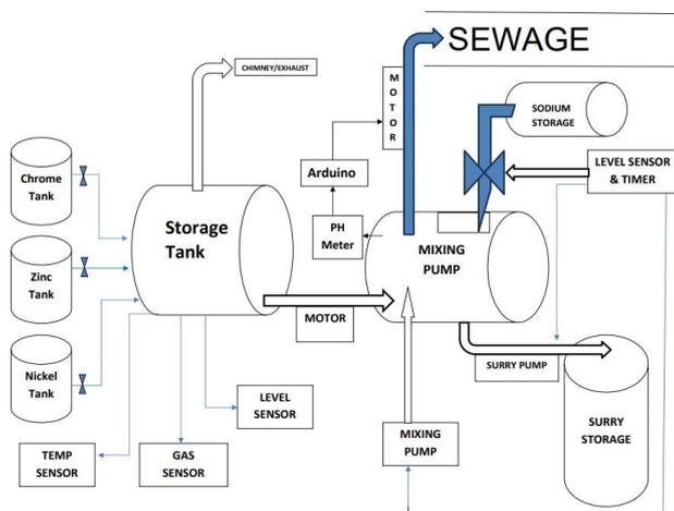
When water is released into ETP plants after washing jobs or electroplated metals or after clearing the chemical tank for maintenance or metals following their electroplating process (such as zinc, nickel, or chrome), a significant volume of water is required for the washing process. However, the water used becomes contaminated with heavy metals, and its pH level becomes either too acidic.
