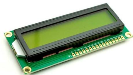
Fig 6: LCD Display
