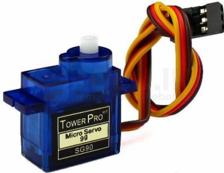
Fig 7: Servo Motor
