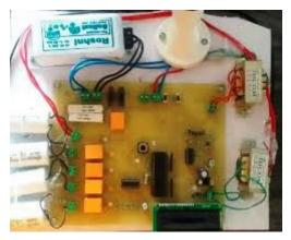
**Fig K. Hardware of Automatic Power Factor Control** Figure shows the whole hardware of Automatic Power Factor Control Unit used for improving power factor. One of the results is discussed below. Figure when inductive load was applied i.e. Choke is used in this case the measured P.F was found to be 0.85 Lagging and the P F is increased to 0.99 by adding capacitor in parallel. The result shows the working and idea of Automatic Power Factor Correct ion by using capacitors.
