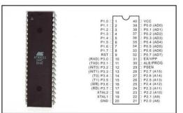
Fig. G. 89S52 Microcontroller and its Pin Diagram
