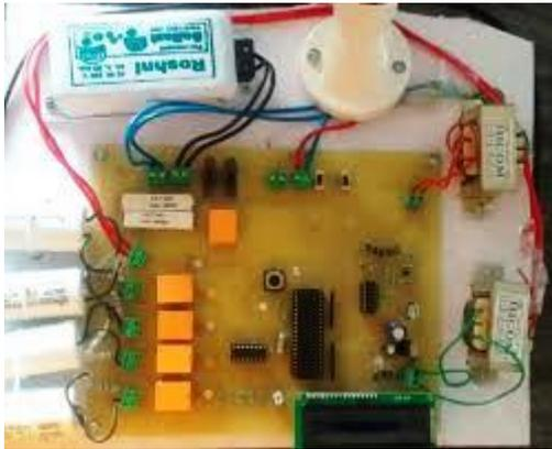
**Fig K. Hardware of Automatic Power Factor Control**
