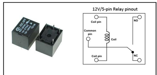
**Fig. H. 12 Volt Relay and its Internal Connection**
