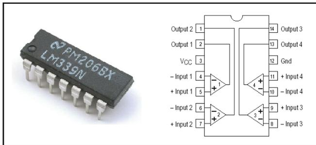
**Fig. C. LM339 IC and its Pin Diagram**
