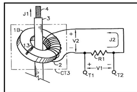
Fig. B. Schematic working of a Current Transformer
