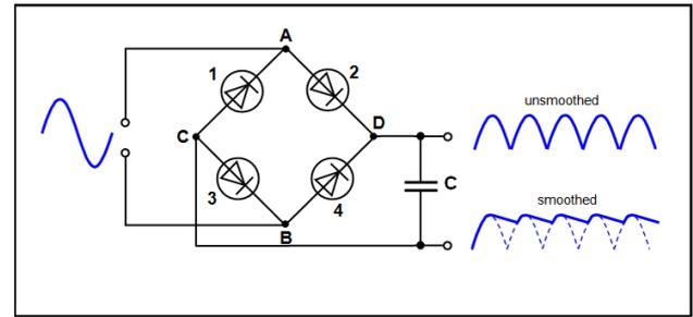
**Fig. D. A Full Bridge Rectifier with Input and Output**
