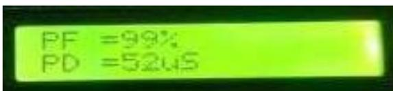
**Fig 5. Showing corrected power factor on LCD**
