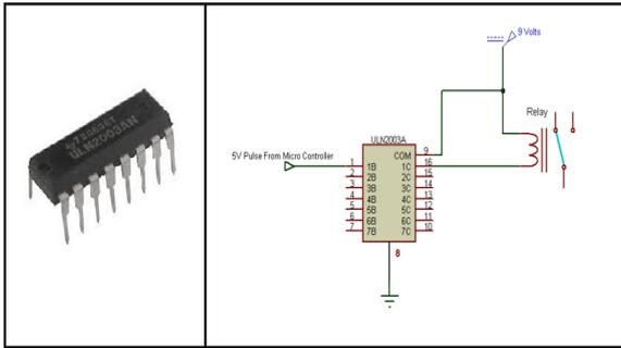
**Fig. I. ULN2003 Relay Driver and its Pin Connection Diagram**
