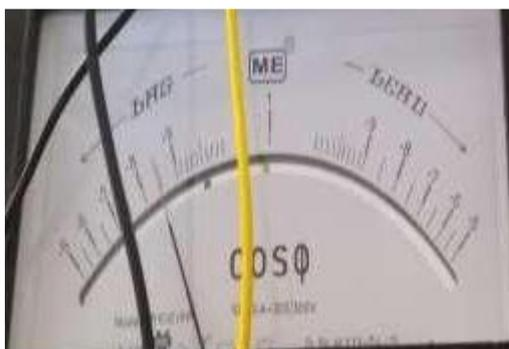
**Fig 4 Measured power factor**
