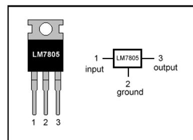
**Fig. E. LM7805 and its Connection Diagram**
