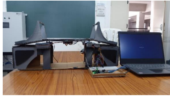
B. Bridge after getting lifted automatically
