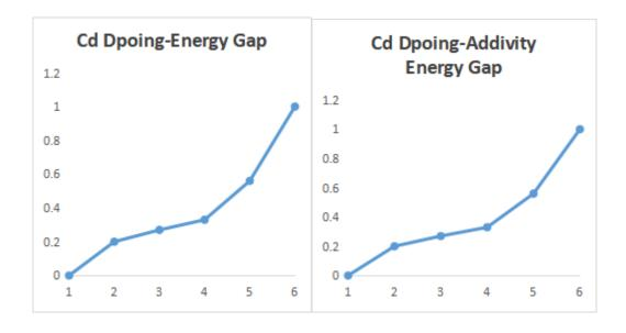
This graph represents Band Energy Gap values of Cd<sub>x</sub>Zn<sub>1-x</sub>Se. Doping of Cd component in a Binary semiconductor like ZnSe and changing the composition of do pant has actually resulted in lowering of Band Energy Gap. Thus effect of do pant increases the conductivity and decreases the Band Energy Gap
