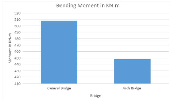
**Fig 3: Comparative analysis of Bending Moment in KN-m**
