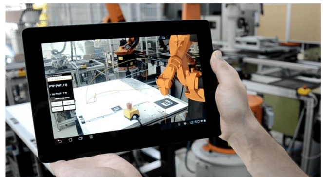
Fig. 4. Mobile marker-based Augmented Reality kinematics
