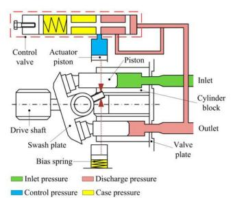
**Figure 1** presents the basic principle of the variable displacement piston pump.
