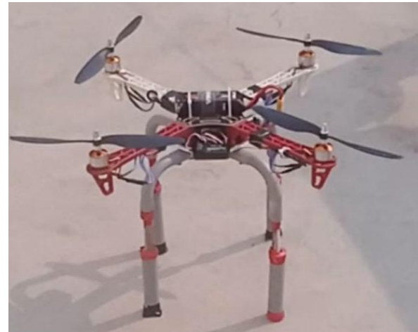
Figure (1) drone with the spring suspension system
