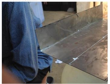
Then the bended plate is screwed to the chassis using hand drilling machine. The support structure is fabricated and it is welded to chassis.
