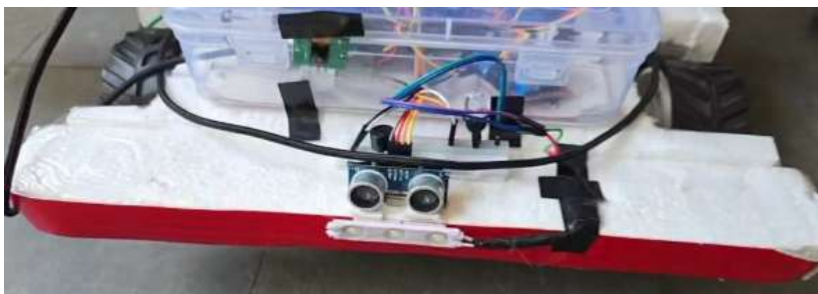
4.9 Front view of the car with ultrasonic sensor and headlights
