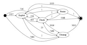
Figure 5 : State diagram of attacker behavior after login
