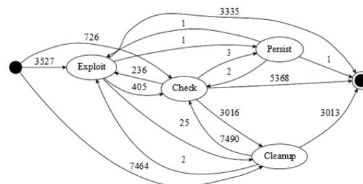
Figure 5 : State diagram of attacker behavior after login
