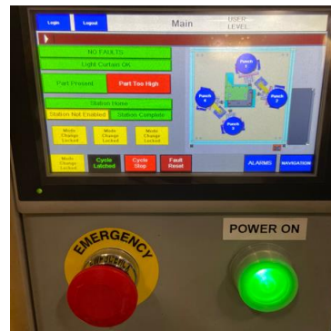
Figure 4: Control Panel Display with Laser Feedback ("Which flags as red 'Part too high' meaning not seated properly all the way in the nest")
