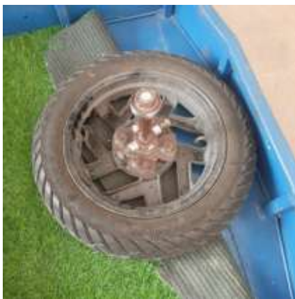
Fig. 14. Failure of Rear Shaft during Physical Testing of EUV within the Campus
