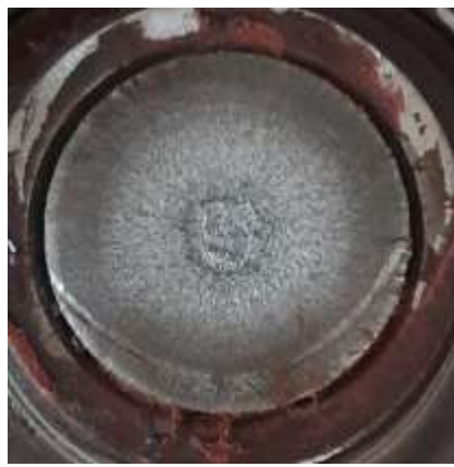
Fig. 14. Failure of Rear Shaft during Physical Testing of EUV within the Campus
