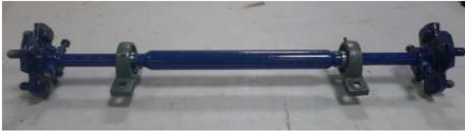
Fig. 15. Redesign and Manufacturing of Rear Shaft of EUV
