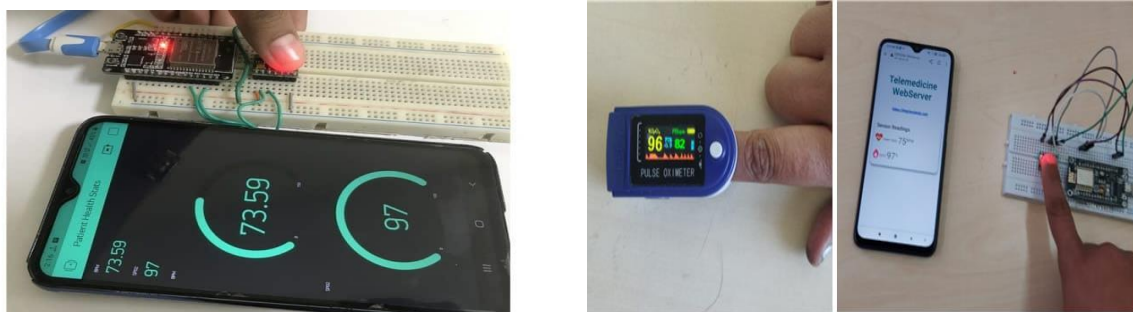
Figure 6 : continuous recording of heart rate, and SpO_2 level on Mobile dashboard The following table shows characteristics of the subjects are considered for experimentation Parameter was recorded during night time in the sleep condition for five hours (11 pm to 4 am).
