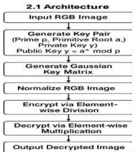
Fig 1. System Architecture of the Proposed Enhanced ElGamal RGB Image Encryption and Decryption Model
