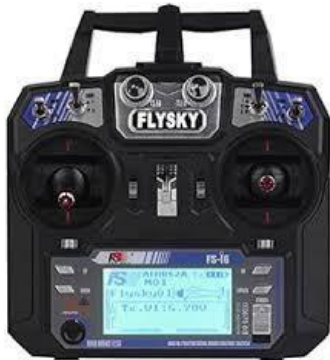
Fig.6 Transmitter (FS-i6 2.4GHz, 6 Channel)
