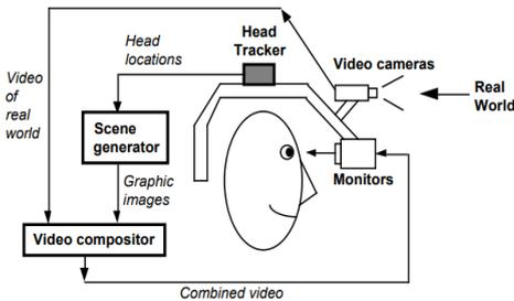
**Figure 4: Virtual Reality Architecture.**
