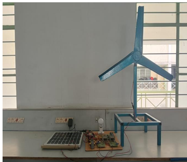
Figure 6. Hybrid Energy System
