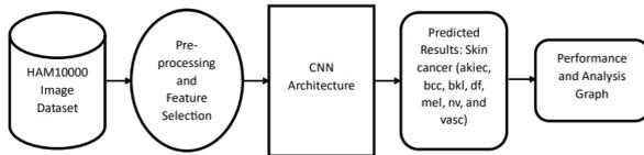
Fig 4.1 System Architecture
