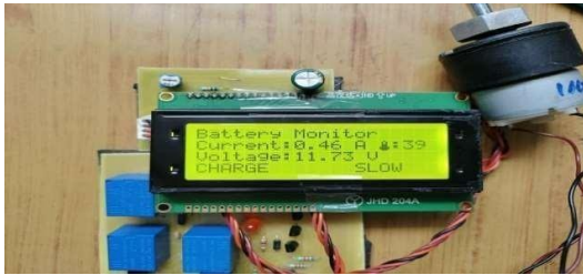
Fig.7 Discharge of battery on the LCD display with voltage reading and temperature display .
