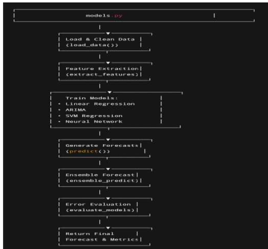
• Figure:4 input Steps for models.py Keeping algorithm logic in a separate module
