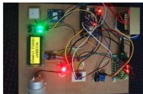
Fig 4.3: Accident Detection and Alert Generation
