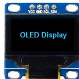
OLED monochrome 128×64 dot matrix display module. The characteristics of this display module are high brightness, self-emission, high contrast ratio, slim/thin outline, wide viewing angle, wide temperature range and low power consumption. OLED's are the future of displays, as they possess some of the greatest advantages over both conventional display technologies of LCD's and LED's.
