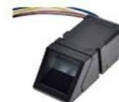
These modules are typically used in safes - there's a high powered DSP chip that does the image rendering, calculation, feature-finding and searching. Connect to any microcontroller or system with TTL serial, and send packets of data to take photos, detect prints, hash and search. You can also enroll new fingers directly - up to 162 finger prints can be stored in the onboard FLASH memory. There's a red LED in the lens that lights up during a photo so you know its working.
