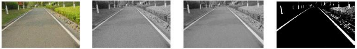
(a) original image (b) grayscale image (c) denoised image (d) binary image
