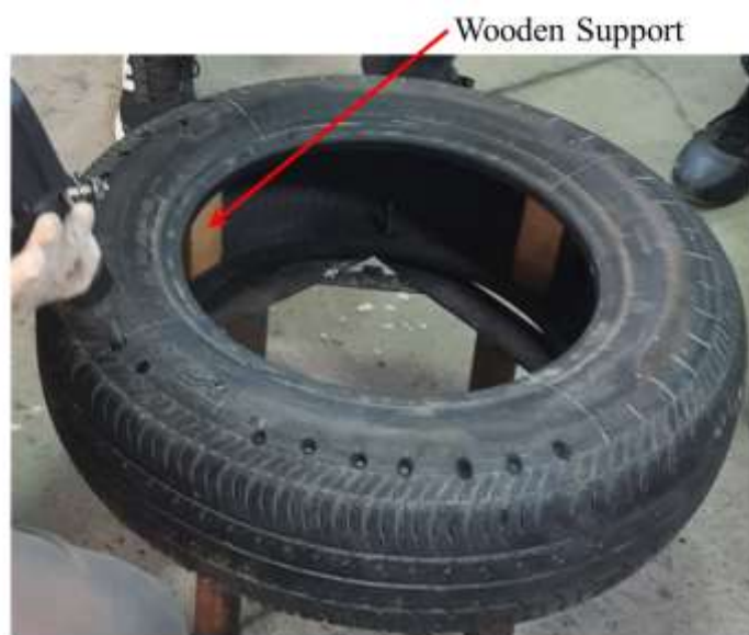
Fig. 1. Wooden Support in Tyres to provide the strength
