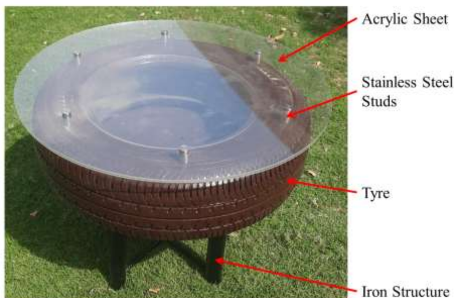
Fig. 5. Table manufactured by Acrylic Sheet, Stainless Steel Studs, Tyre and Iron Structure
