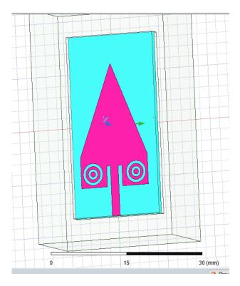
Figure 2: Triangular patch-CSRR structure
