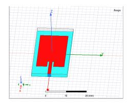
Figure 1 : Basic microstrip patch antenna
