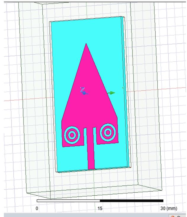
Figure 2: Triangular patch-CSRR structure
