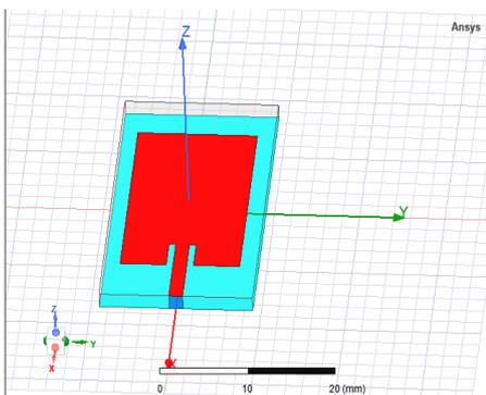
Figure 1 : Basic microstrip patch antenna
