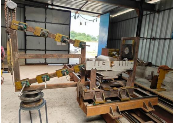
Fig. 5.1 Fabrication of Creel Stand
