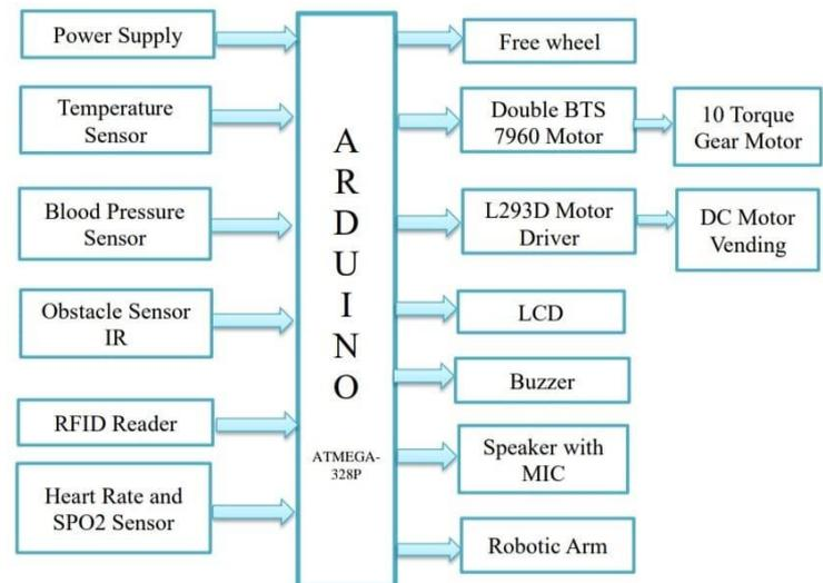
Figure 1: Block diagram of Patient monitoring Humanoid Robot For Pandemic Situations.
