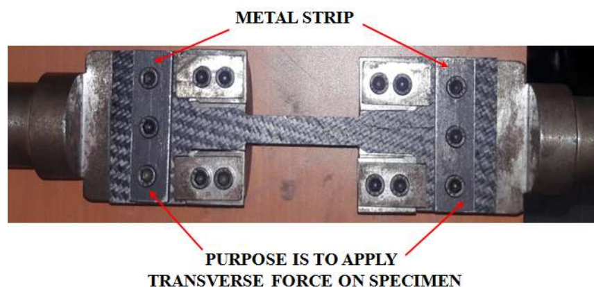
Fig. 11. Modified Assembly of Fixture and CFRC Specimen
