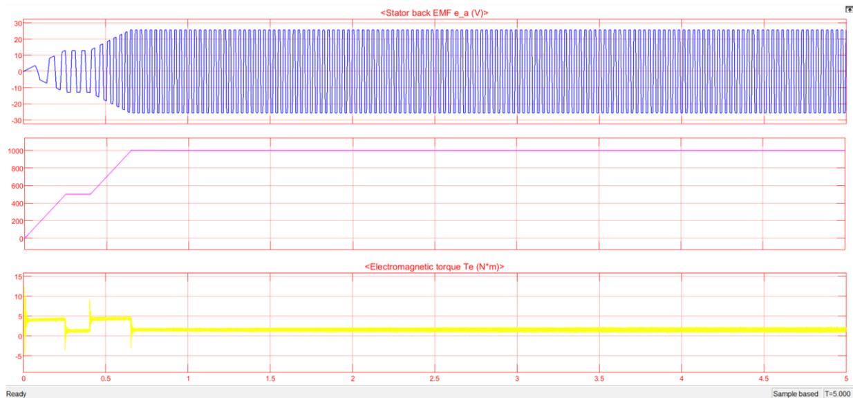
**Fig:10:** Output waveform for BLDC motor torque and speed and EMF.
