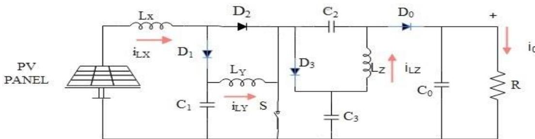
**Fig:4:** Circuit diagram for MSC converter mode I.
