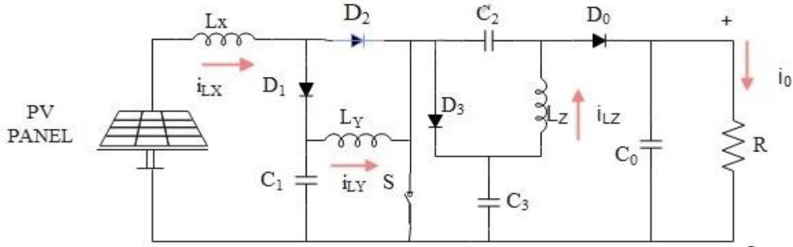
**Fig:5:** Circuit diagram for MSC converter mode II
