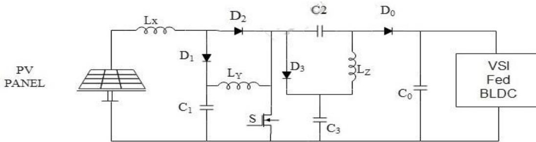
**Fig:3:** Circuit Diagram for Proposed Modified Sepic Converter.
