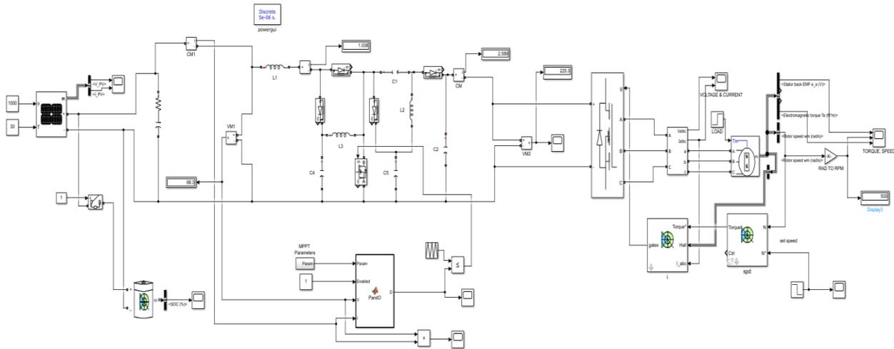
**Fig:6:** Simulation circuit diagram for MSC Converter.
