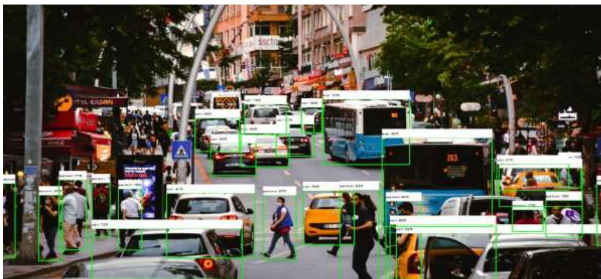
Fig: Object Detection on Images with Bounding Boxes
