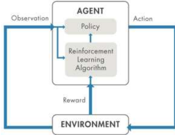
Figure 1: Basic Reinforcement Learning Framework showing agent-environment interaction.
