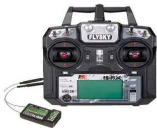
Figure - 2 : Transmitter & Receiver connection
