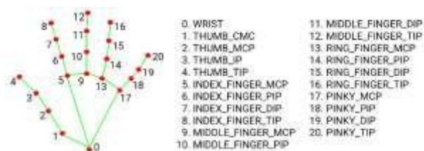
Fig 7.1 Hand landmark detection using MediaPipe Result And Discussions
