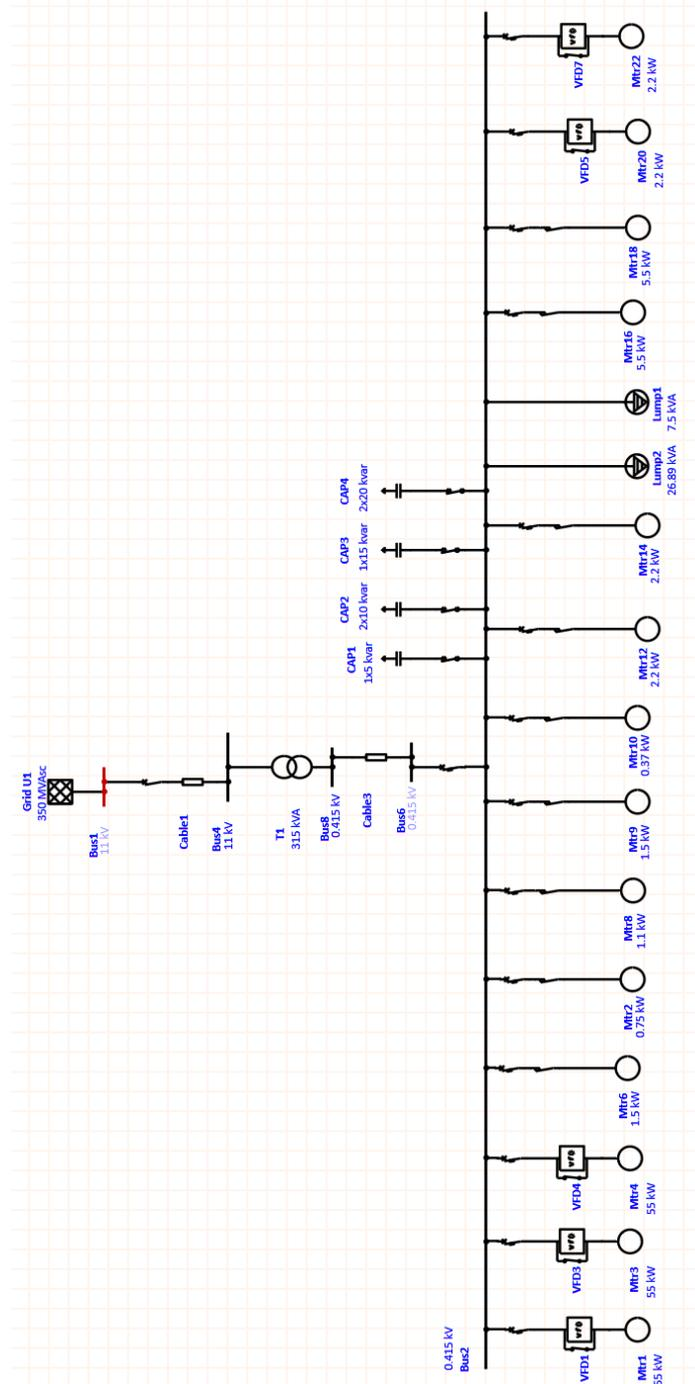
Fig-2: One Line Diagram Indicating the Various Components of the Distribution System
