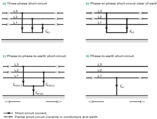
Fig-1: Different types of short-circuits and their currents. The direction of current is chosen arbitrarily as per IEC 60909.
