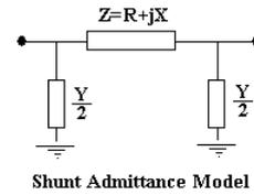
Fig: 2 Shunt Admittance Model
