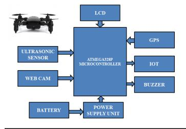
Fig -1Main Parts Drone for Food Delivery
