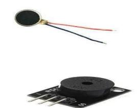
This buzzer will be used to generate sound if any alert happens near the stick. The buzzer is a small device that makes sound when it gets electrical signals. It beeps when the sensor finds an obstacle and the ESP32 sends a signal to the buzzer. This sound helps alert the person about something in the way. The buzzer works even if the device is not connected to a phone.
