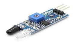
An Infrared Sensor (IR Sensor) is a radiation sensitive optoelectronic component with a spectral sensitivity in the infrared wavelength extend 780 nm ... 50  $\mu$ m. IR sensors are now broadly used in movement detectors, which are utilized in building services to switch on lights or in alarm systems to detect unwelcome guests.
