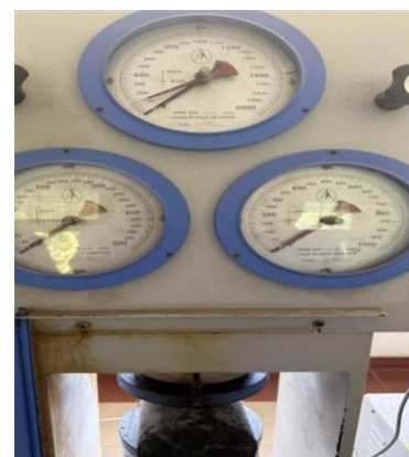
Fig.8: Test Set Up for Split Tensile Strength (Cylinder)
