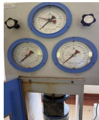
Fig. 7: Test Set Up for Testing Compressive Strength (Cube)
