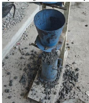
Fig. 11: Test Set Up for Compaction Factor Test
