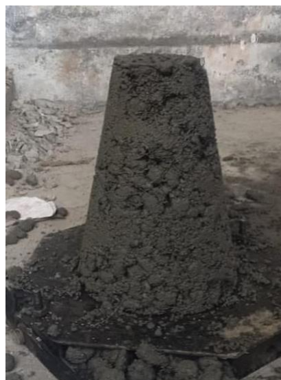
Fig. 10: Test Set Up for Slump Cone Test
