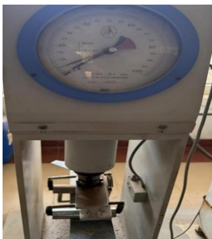
Fig.9: Test Set Up for Flexural Strength (Beam)
