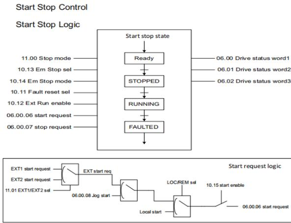
**Jog Start** - Jog start has two signal sources; they are respectively as 10.08 Jog1 start (Jog1 start) and 10.09 Jog2 start (Jog2 start). When the two jog commands are effective at the same time, the jog command JOG1 is prioritized. User can enable or disable the jog function with the parameter
